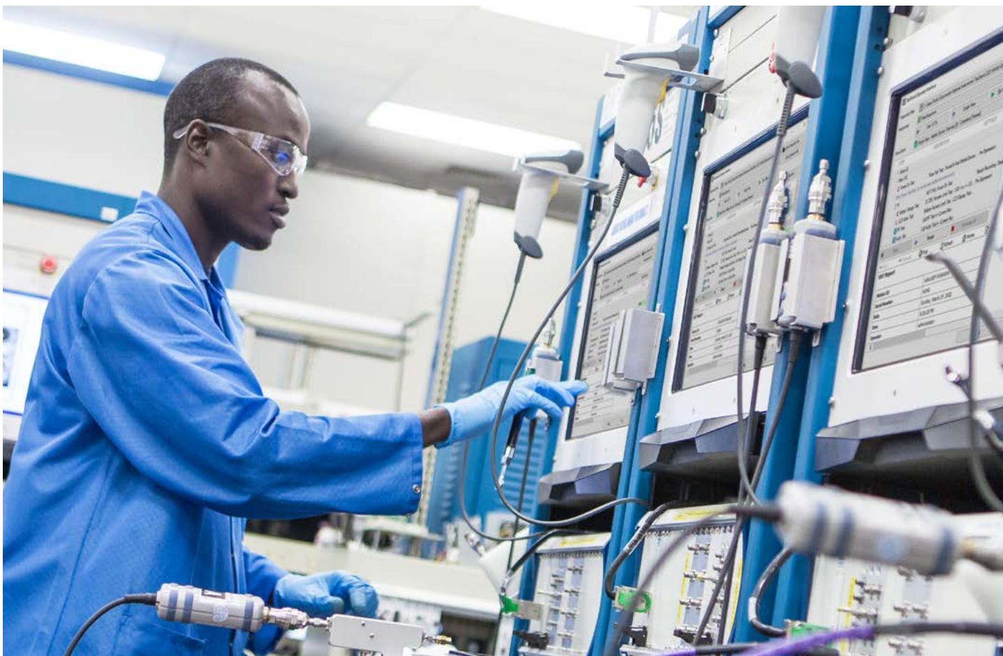
NI PXI used with TestStand in an RF manufacturing test system
