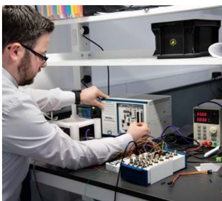
PXI used for benchtop validation system
